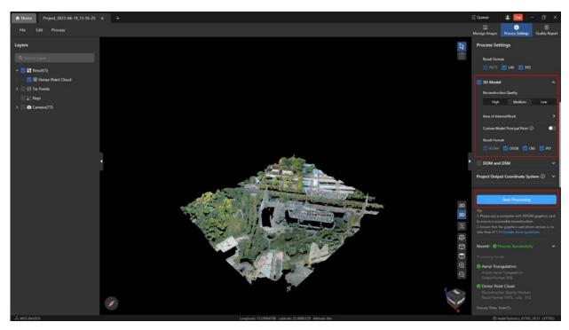
During processing, you can click the [**Stop**] button to stop processing, and modify the reconstruction quality or result format before processing.
