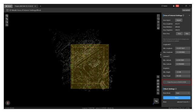
After drawing the area of interest in 2D mode, click the [Copy the area to 3D Model] button at the bottom of the [Area of Interest Settings] column to apply the drawn area of interest to the area of interest of the 3D model.
