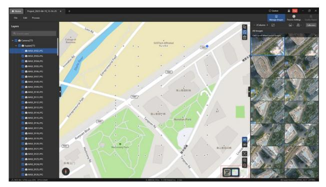
When the mouse moves in the 2D view, the coordinate value of the current mouse position will be displayed in the bottom coordinate system bar below the view. For details, please refer to section 4.3 of this chapter.
