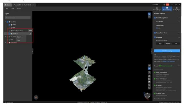
The export results support the selection of B3DM, OSGB, OBJ, and PLY formats. If the corresponding result format is not checked when processing the 3D model, the corresponding format cannot be selected when exporting.
