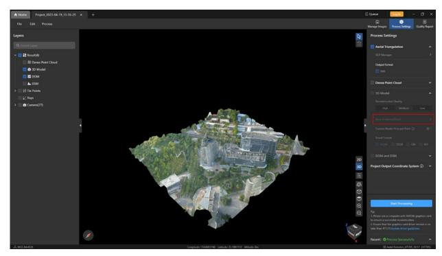
When logging in to an Autel Mapper account, and the account is within the validity period, click the [Area of Interest /Block] button under the [3D Model] in the [Process Settings] page to enter the [3D Mode Area of Interest Settings/Block] page, in this page model block settings can be changed.
